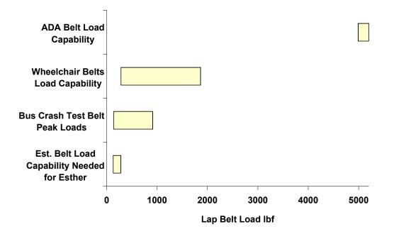
**Figure 1.** Summary of lap belt capabilities (ADA, Karg tests), peak loads recorded in crash tests (UMTA tests), and the estimated belt load required to provide the restraining force needed to keep Esther in her wheelchair during the vehicle motion event.
